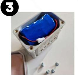
VOUS APERCEVEZ LA PILE CONNECTER LA PILE AVEC LA FICHE DE CONNEXION DANS LE DELTA R ATTENTION AU SENS DE BRANCHEMENT
